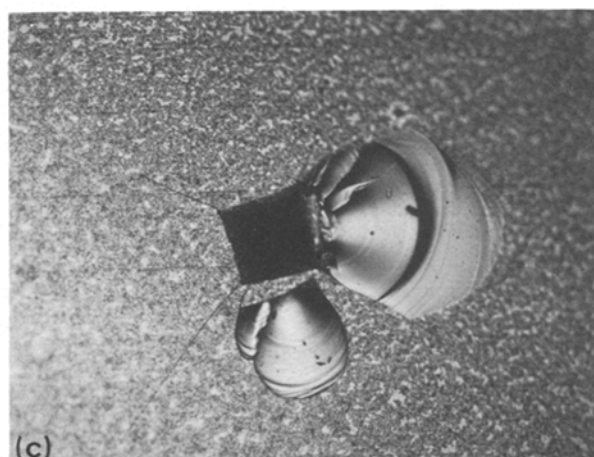
Figure 2 Typical photograph of Vickers indenter marks representing all the arsenic–selenium compositions studied: (a) load 100 g; (b) occasional formation of two cracks from the indenter diagonal (c) load 800 g.
